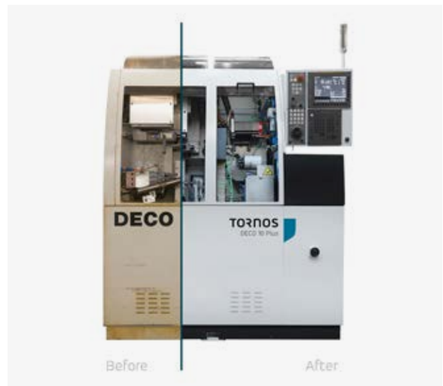
Tornos DECO 2000 machine before and after retrofitting
